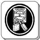
Prior to any repair works on the dust collector and its drives, secure the dust collector against unintentional switching-on. Pull out the mains plug in order to do this.
